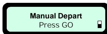
Figure 5.2 – LCD Display on Robomow when docked and NO Weekly Program is set OR the 'Auto Depart' function is turned off
