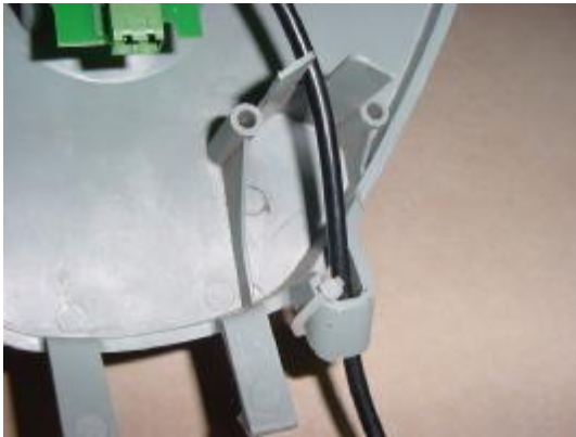
Figure 1.18 Routing the Power Supply cord into the cover
