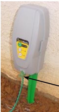
Figure 1.35 – Perimeter Switch with mounting stake attached
