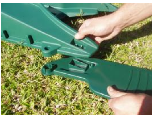
Figure 1.24a – Wheel support alignment
