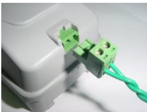
Figure 1.33 – Plug the plot connector into the Perimeter Switch
