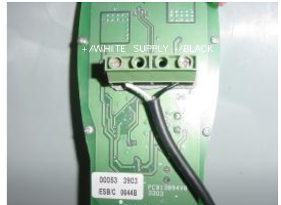
Figure 1.19 Power Supply Cord Track through the cover
