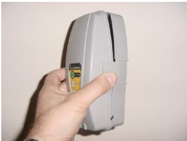
Figure 1.31 - Squeeze to remove cover
